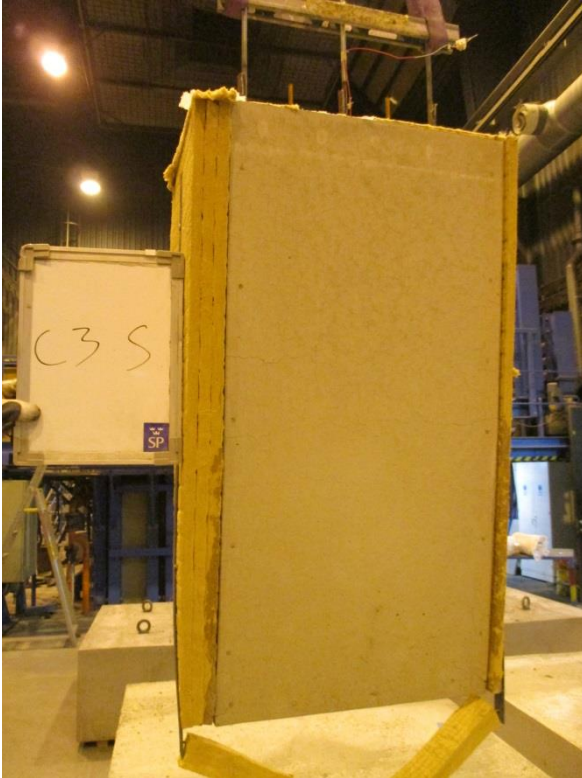
Figure A72. Test specimen Wedge-Slab 24: 1000x500-50-300 Mix 3 0.40-0.0kgPP after the test.
