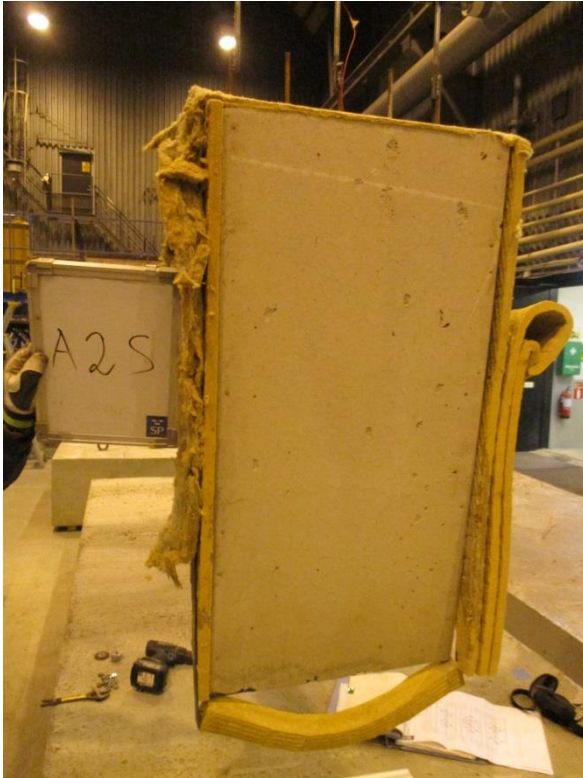
Figure A57. Test specimen Wedge-Slab 26: 1000x500-50-300 Mix 1 0.33-1.0kgPP after the test.
