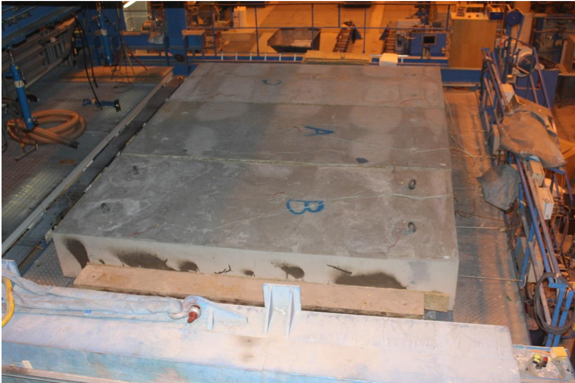
Figure A96. Test specimens on the furnace during the test.
