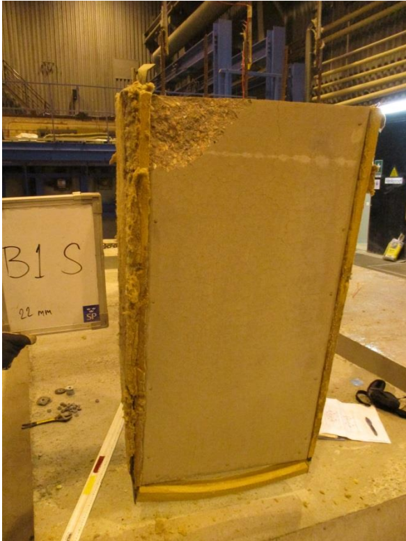
Figure A61. Test specimen Wedge-Slab 19: 1000x500-50-300 Mix 2 0.33-0,0kgPP after the test. Maximum spalling: 22 mm
