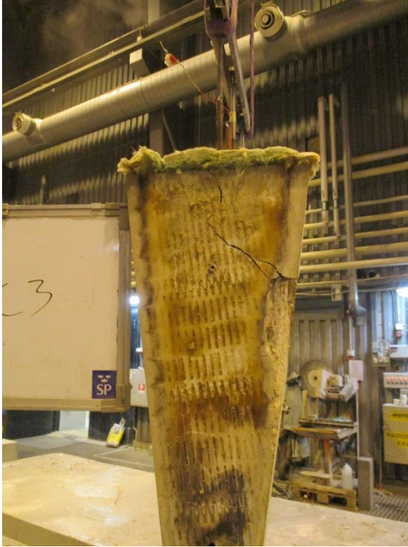
Figure A74. Test specimen Wedge-Slab 24: 1000x500-50-300 Mix 3 0.40-0.0kgPP after the test. Side view.
