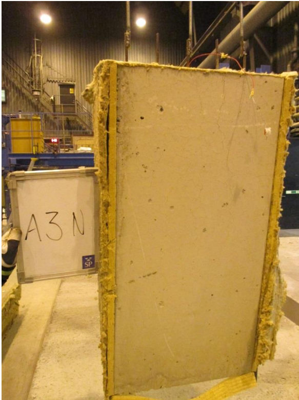
Figure A60. Test specimen Wedge-Slab 27: 1000x500-50-300 Mix 1 0.33-1.0kgPP after the test.
