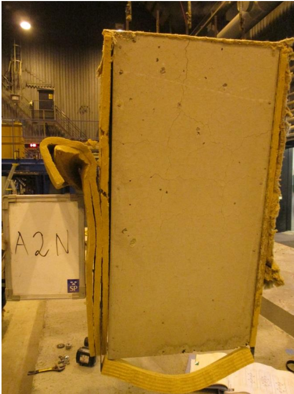
Figure A58. Test specimen Wedge-Slab 26: 1000x500-50-300 Mix 1 0.33-1.0kgPP after the test.
