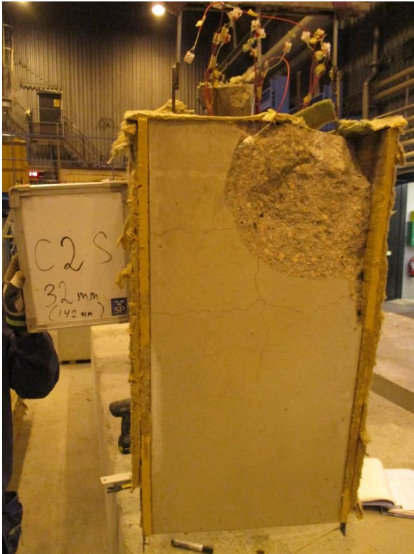
Figure A70. Test specimen Wedge-Slab 23: 1000x500-50-300 Mix 3 0.40-0.0kgPP after the test. Maximum spalling: 32 mm
