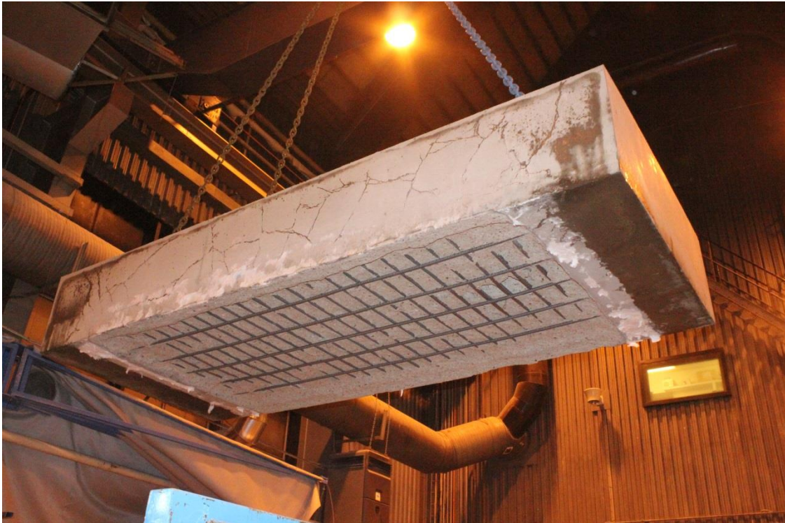
Figure A98. Test specimen Large slab 28: 4000x1670-600 Mix 2 0.33-0,0kgPP after the test.
