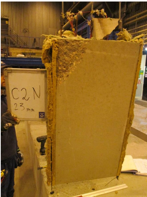
Figure A71. Test specimen Wedge-Slab 23: 1000x500-50-300 Mix 3 0.40-0.0kgPP after the test. Maximum spalling: 23 mm
