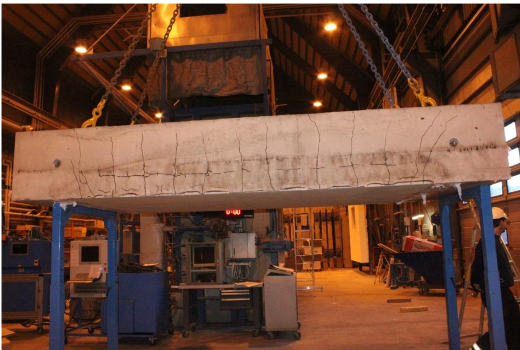
Figure A103. Test specimen Large slab 30: 4000x1670-600 Mix 1 0,40-1,0kgPP after the test.
