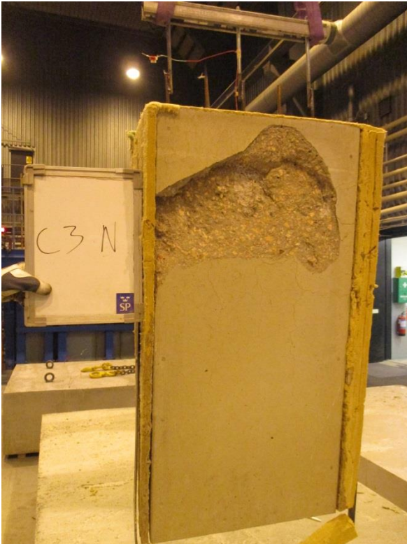
Figure A73. Test specimen Wedge-Slab 24: 1000x500-50-300 Mix 3 0.40-0.0kgPP after the test. Maximum spalling: 42 mm
