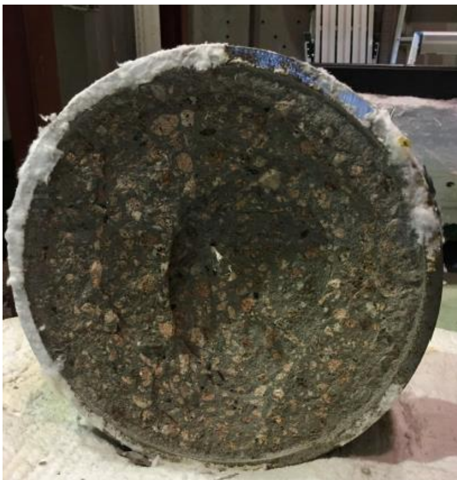
Figure A104. Test specimen MixB,1 after the fire test.
