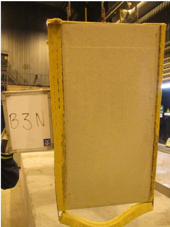
Figure A67. Test specimen Wedge-Slab 21: 1000x500-50-300 Mix 2 0.33-0.0kgPP after the test.
