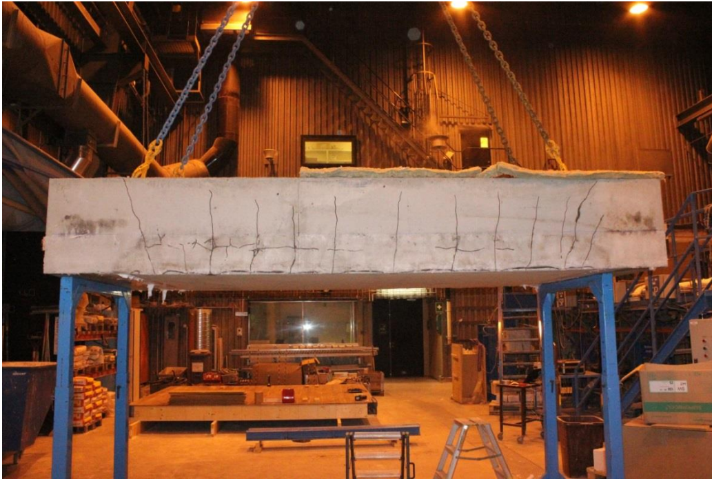
Figure A102. Test specimen Large slab 30: 4000x1670-600 Mix 1 0,40-1,0kgPP after the test.
