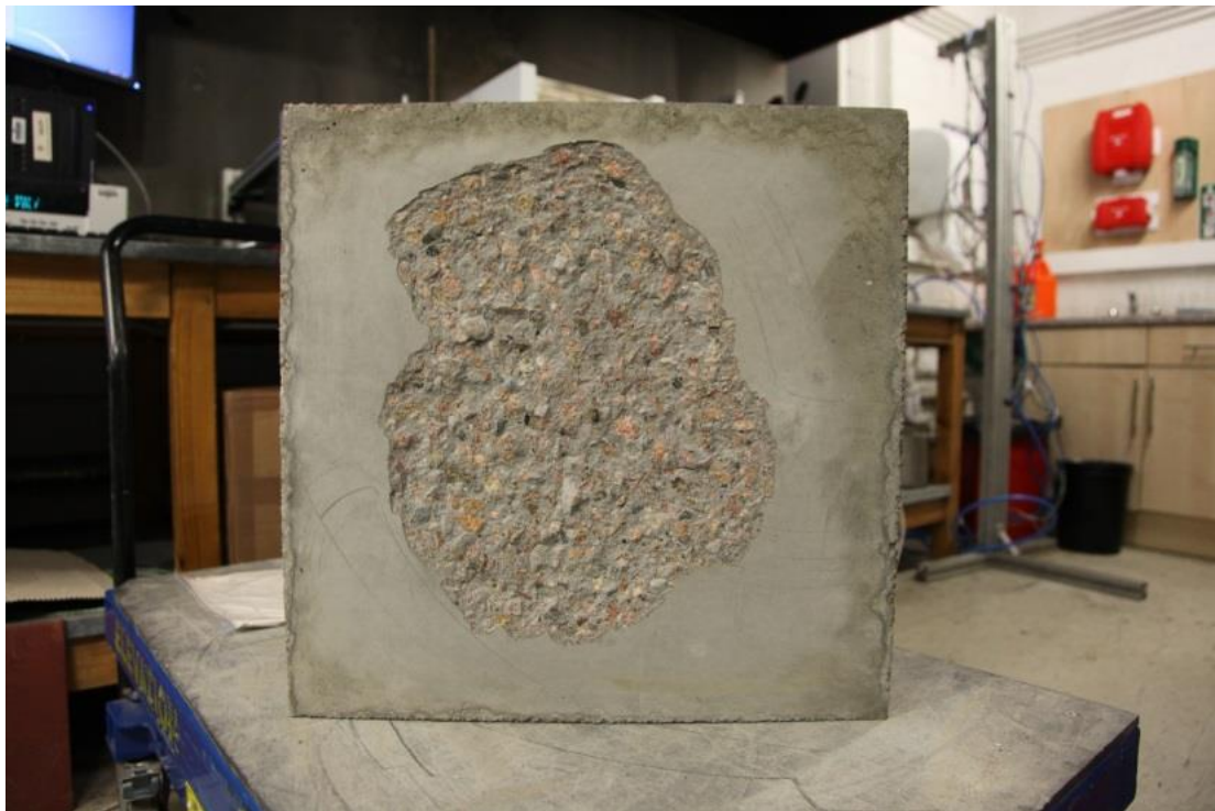
Figure A105. Test specimen Mix3,3 after the fire test.
