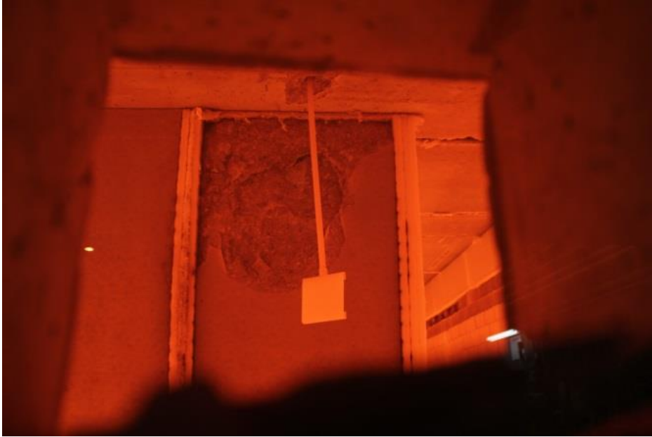
Figure A85. Test specimen Wedge-Slab 21: 1000x500-50-300 Mix 2 0.33-0.0kgPP during the test.
