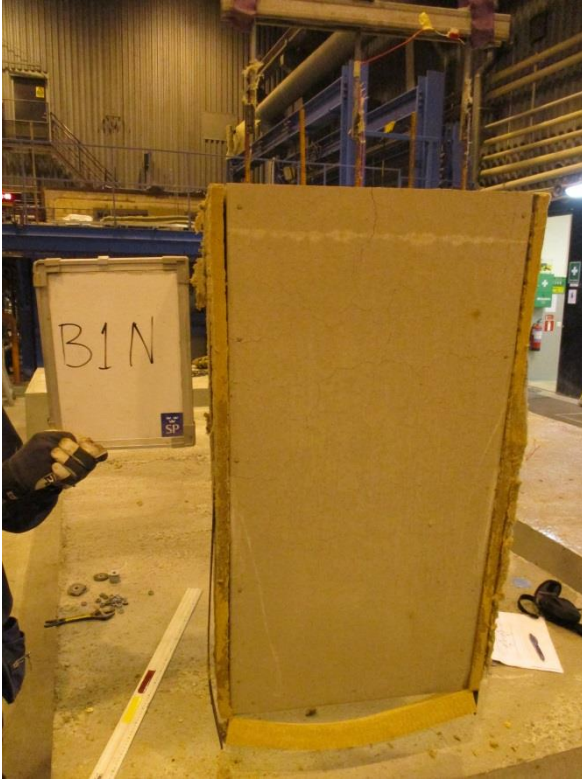
Figure A62. Test specimen Wedge-Slab 19: 1000x500-50-300 Mix 2 0.33-0,0kgPP after the test.
