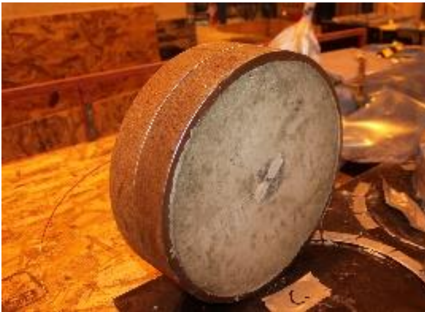
Figure 4. Concrete moulded in steel pipes, Gunma University type.
