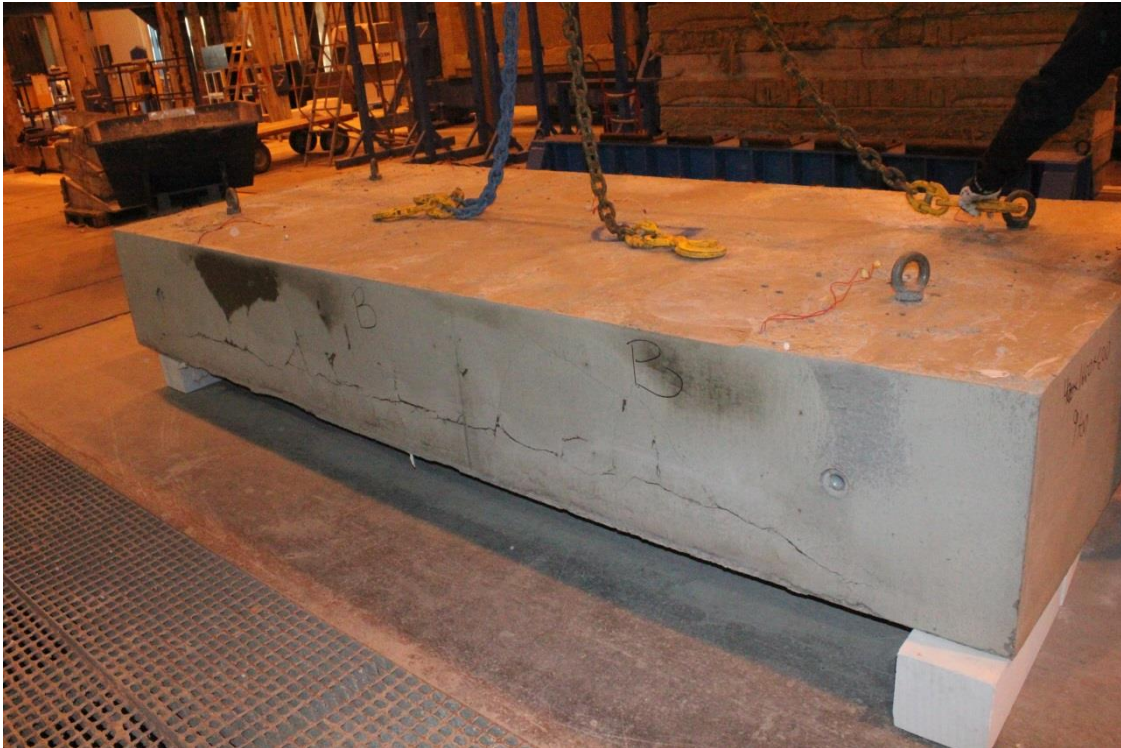
Figure A100. Test specimen Large slab 28: 4000x1670-600 Mix 2 0.33-0,0kgPP after the test.
