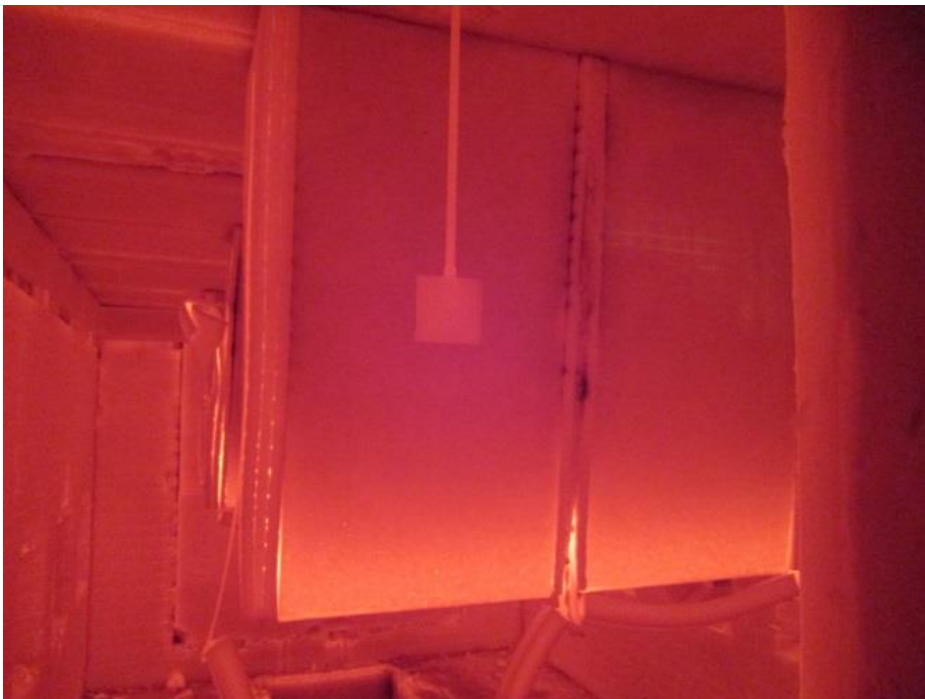
Figure A84. Test specimens Wedge-Slab 22: 1000x500-50-300 Mix 3 0.40-0.0kgPP, Wedge-Slab 19: 1000x500-50-300 Mix 2 0.33-0,0kgPP during the test.
