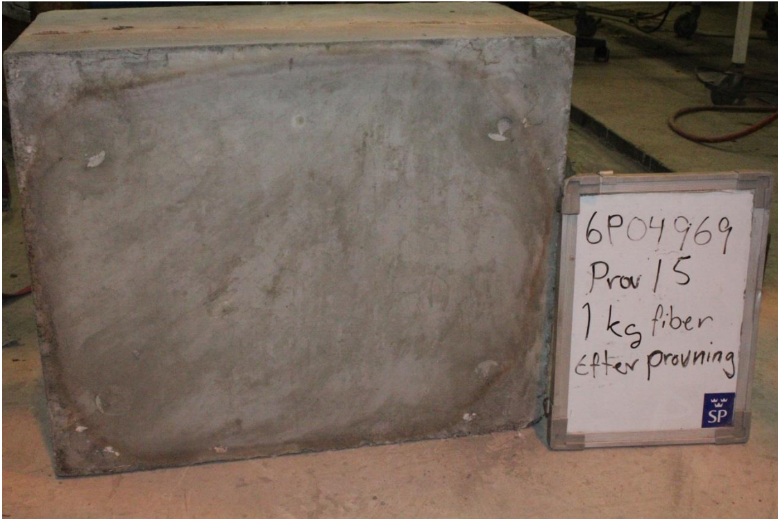
Figure A146. Test specimen after the test.
