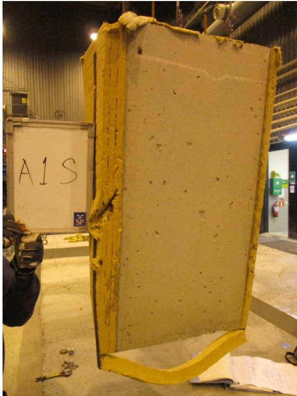
Figure A55. Test specimen Wedge-Slab 25: 1000x500-50-300 Mix 1 0.33-1.0kgPP after the test.
