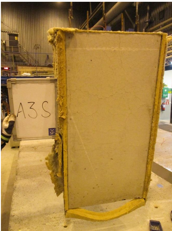
Figure A59. Test specimen Wedge-Slab 27: 1000x500-50-300 Mix 1 0.33-1.0kgPP after the test.
