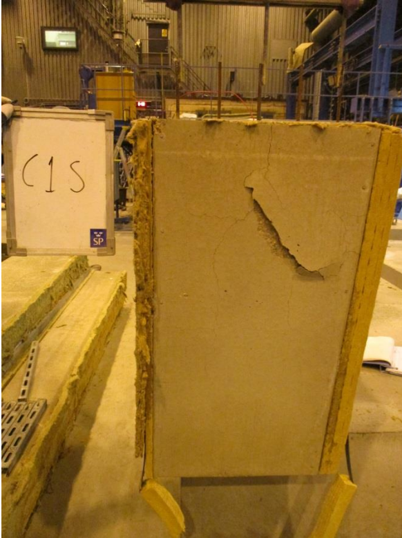
Figure A68. Test specimen Wedge-Slab 22: 1000x500-50-300 Mix 3 0.40-0.0kgPP after the test.
