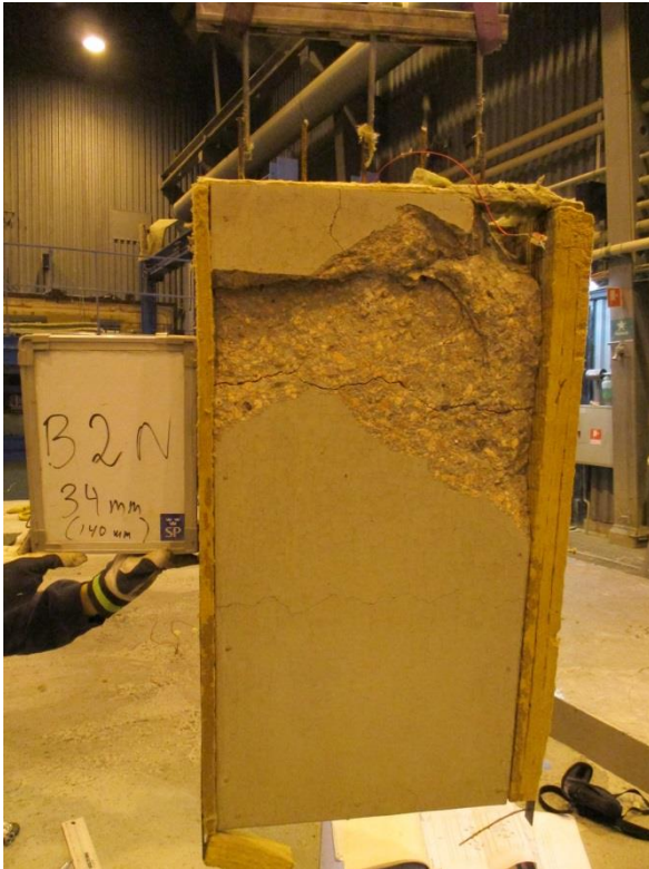
Figure A64. Test specimen Wedge-Slab 20: 1000x500-50-300 Mix 2 0.33-0.0kgPP after the test. Maximum spalling: 34 mm
