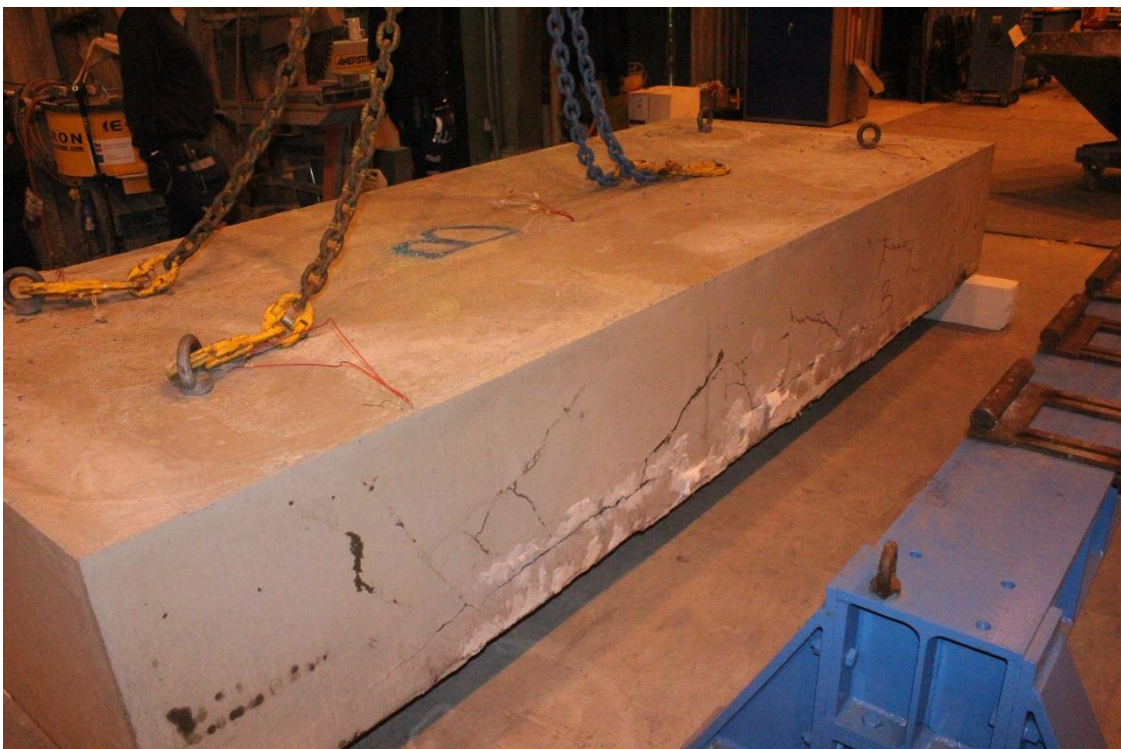
Figure A99. Test specimen Large slab 28: 4000x1670-600 Mix 2 0.33-0,0kgPP after the test.
