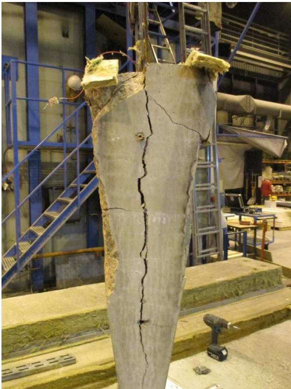
Figure A65. Test specimen Wedge-Slab 20: 1000x500-50-300 Mix 2 0.33-0.0kgPP after the test. Side view.
