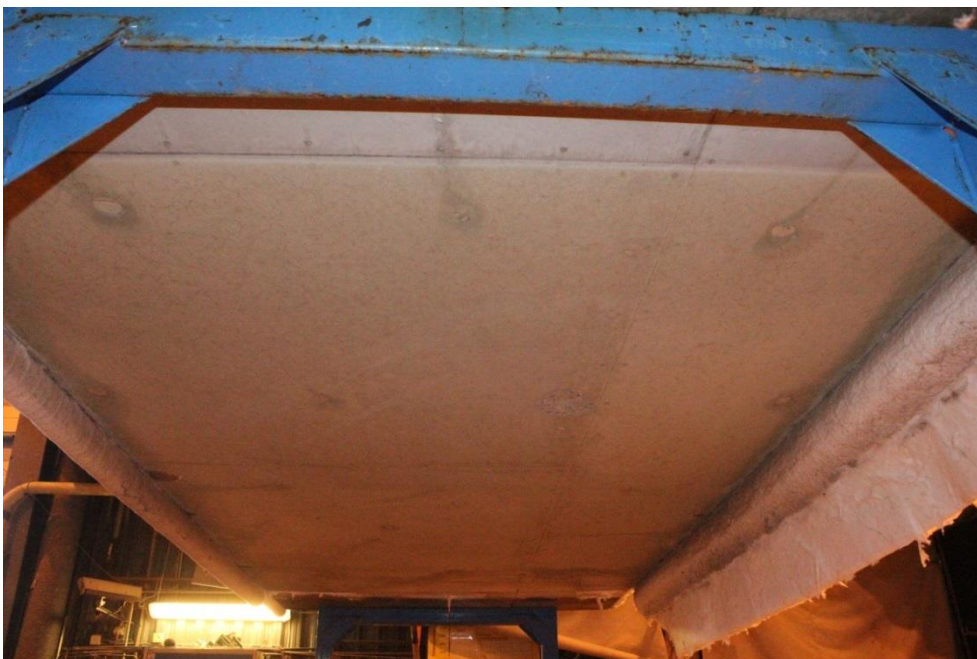
Figure A101. Test specimen Large slab 30: 4000x1670-600 Mix 1 0,40-1,0kgPP after the test.
