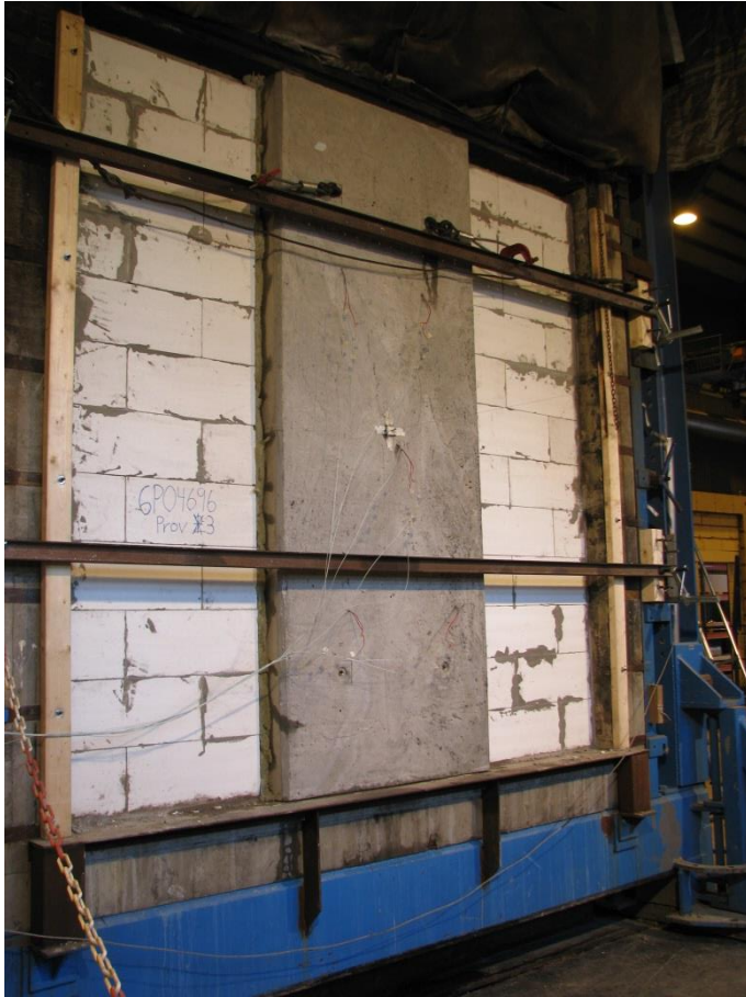
Figure A166. The slab after the test. The slab is cracked on the sides. Water is coming out from the cracks.
