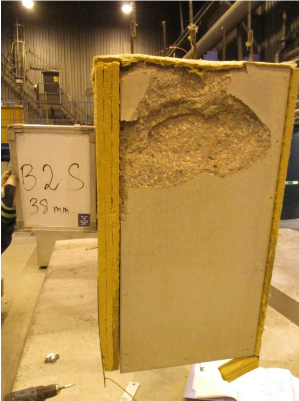
Figure A63. Test specimen Wedge-Slab 20: 1000x500-50-300 Mix 2 0.33-0.0kgPP after the test. Maximum spalling: 38 mm
