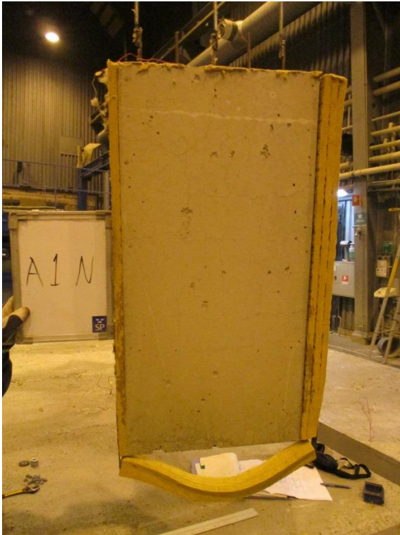
Figure A56. Test specimen Wedge-Slab 25: 1000x500-50-300 Mix 1 0.33-1.0kgPP after the test.
