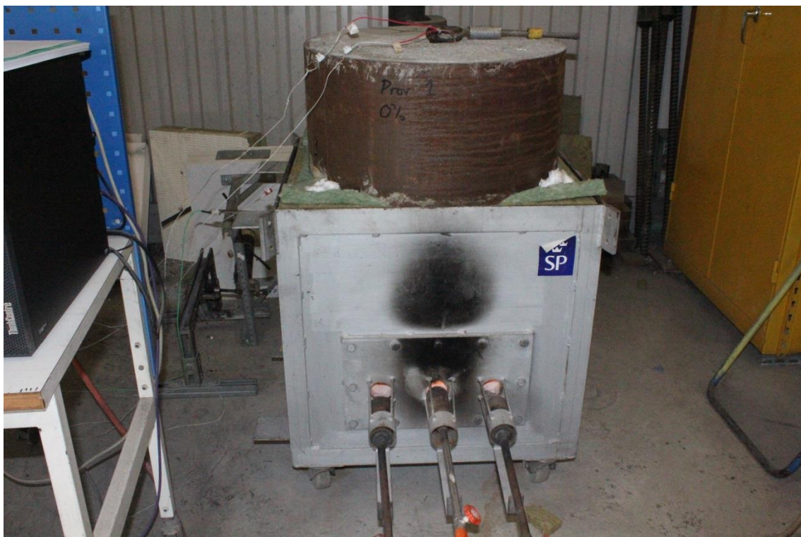
Figure A106. Test specimen during the test.
