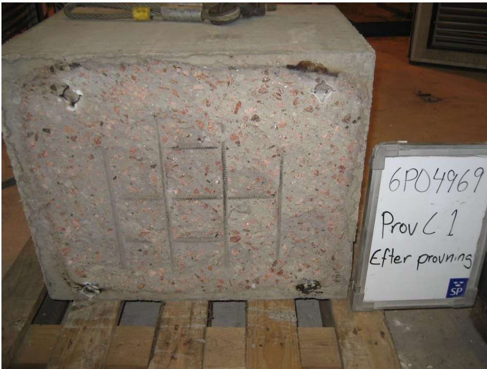
Figure A20. Test specimen after the test.
