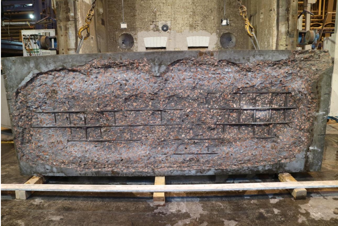
Figure A162. Test specimen after the test. The whole surface is spalled to the depth of the reinforcement
