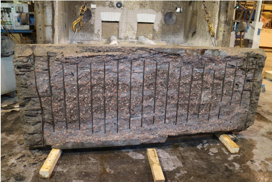
Figure A152. Test specimen after the test. The whole surface is spalled to the depth of the reinforcement.
