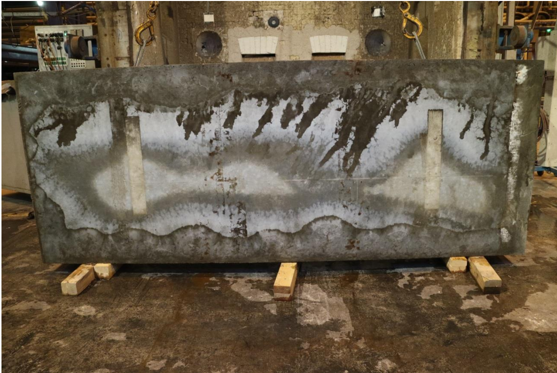
Figure A171. Test specimen after the test. No spalling was observed.
