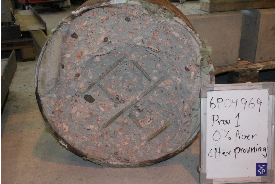
Figure A107. Test specimen after the test.
